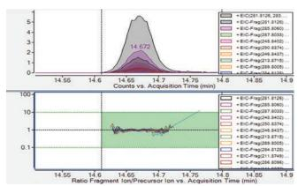
In the **MassHunter Qualitative Analysis software**, the *Compound Details view* of the All lons workflow allows for quick review of the screening. This view includes the Overlayed Extracted Ion Chromatograms (top) and the Coelution Plot (bottom) for the fragment ions of a pesticide. Verifying the coelution of the compound fragments is a critical part of compound confirmation.
